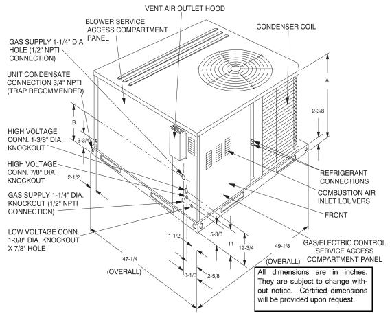
FIGURE 7 - UNIT DIMENSIONS - FRONT
